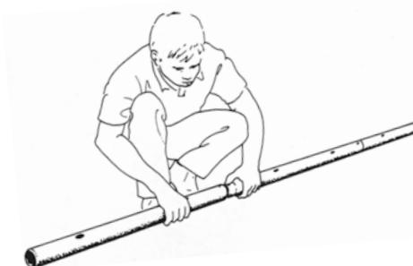
3. Assemble the top tube, starting with 1 pole **A**, as many poles **B** as necessary to make up the length (following the plan) and ending with 1 pole **C**.
